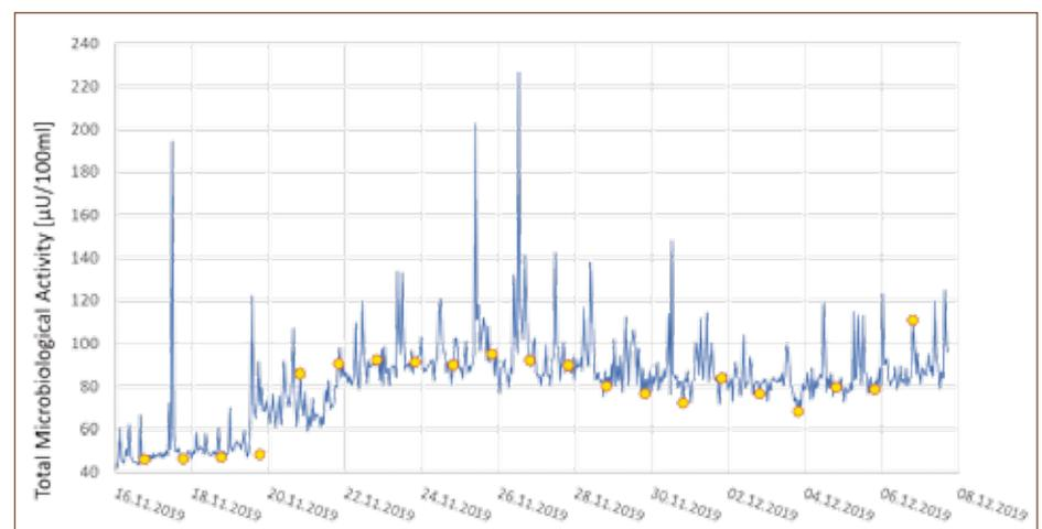
**Table 1** Example of a timeline of microbiological activity in a drinking water pipeline; blue line: measured course of microbiological activity, yellow dots: two manually taken samples per day
