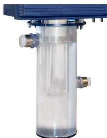
CMS5000 rapidly analyzes VOCs in water using a modified EPA purge and trap concentrator protocol. The state-of-the-art SituProbe™ purges VOCs from water and collects them on a concentrator prior to GC analysis. There is no need for sample pre-treatment or filtration. Since the water condition does not affect the system's
